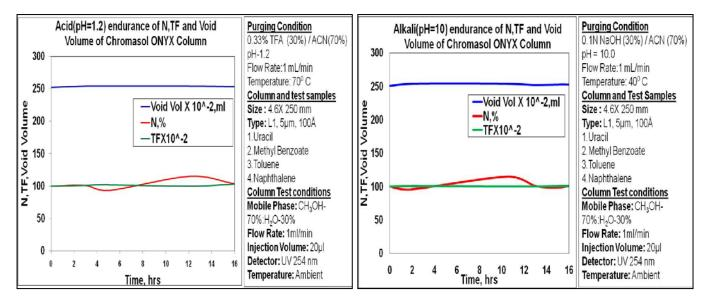
CHROMASOL ONYX is tested to have good acid and alkali stability in the range 1.2-10 and is illustrated in the Figures where in minimal changes in N and TF are noticed with both the variations being parallel to the time axis up to 16 hrs under aggressive test conditions.
